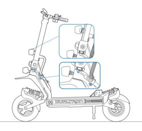
③Install the screws for headlight/damper with the included multitool or An M6 Allen key.
