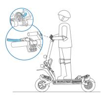
**4.** Slow down by releasing the throttle and squeezing brake levers.
