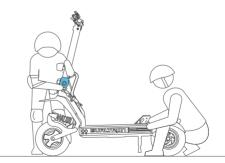
Lift up the bottom of the front fork and rear foot pedestal to carry if necessary. Make sure the scooter is carried by two or more people. Risk of pinching!
