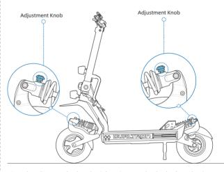
Turn the adjustment knob to the right to increase the shock rebound resistance. Turn the adjustment knob to the left to decrease the shock rebound resistance. Note: The shock is set to the default position before leaving the factory. Please follow the steps above to adjust it according to your riding habits.
