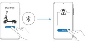
Click "Search vehicle" and pair with your scooter. \* The scooter is connected to the Dualtron app when the Bluetooth symbol lights up. Method 2
