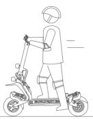
Stand on the footboard with one foot and push off with the other foot to start gliding. \*Make sure you have disabled SAFE mode.(SAFE mode setting via Dualtron app.Deactivate safe mode by squeezing brake lever.)
