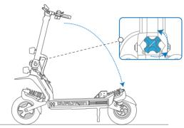
Unscrew the folding knob and M8 screws, then fold the steeing tube. Risk of pinching!
