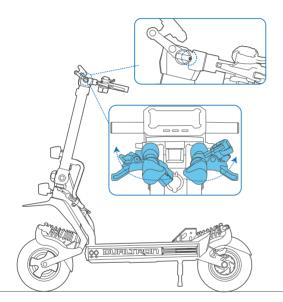
Unfold the handlebars, slide the folding handle lock into position to fix the handle firmly. During use, if the handle is slightly shaken, please unscrew the adjustment screw a little.
